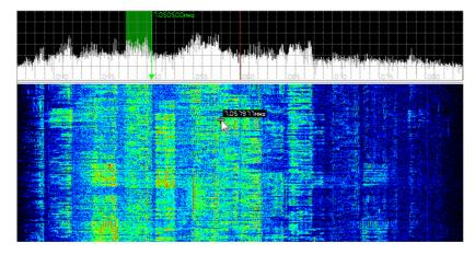
Monitor existing signals within the visible 48KHz width, and pick it up by just pointing and clicking on the signal.
